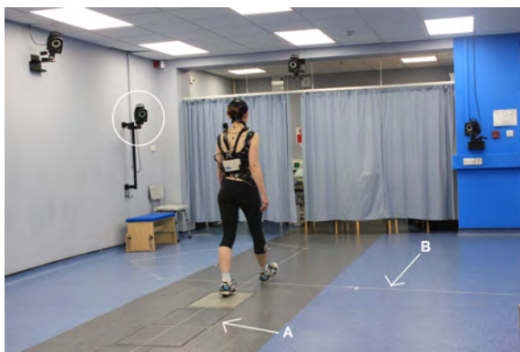
Figure 2.5: Participant crossing force plates (A) in Oxford Gait Laboratory wearing K4b2 breath analysis kit and passive motion tracking markers. Four Vicon motion tracking cameras (e.g. circled) are shown. Participants were asked to follow the white string (B), laid in a figure eight pattern, to maintain continuous walking.
