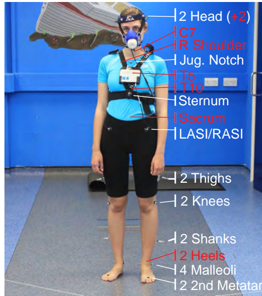
Figure 2.6: Location of motion tracking markers on a test subject during NOC II tests. Hidden markers indicated in red.
