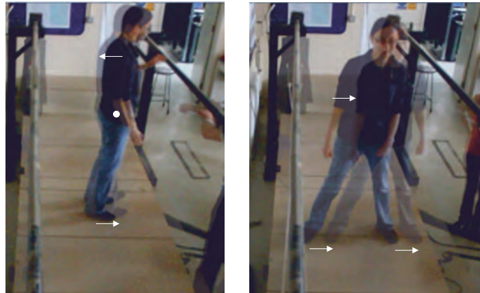
Figure 7.11: Fixed-in-space (FIS, left) versus fixed-to-base (FTB, right) stability strategies for standing. In FIS standing, subject allows body to rotate about CoM as bridge moves. In FTB standing, whole body moves as a ‘rigid’ unit along with the bridge.
